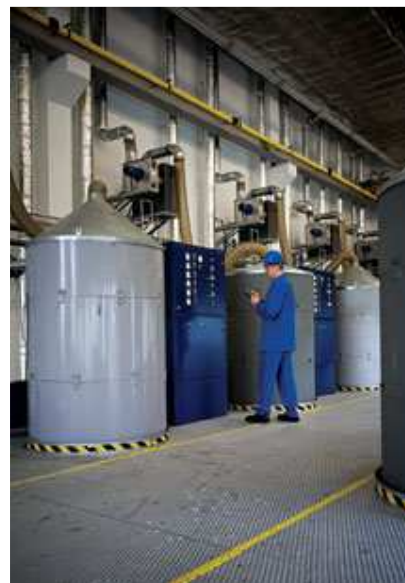
Photo: Robert Laska Ammono's Autoclaves: In a single run, they now produce over 70 2-inch crystals of gallium nitride.
